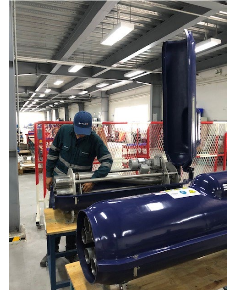
Selector valve inspection
